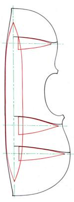
As you can expect the wood to sink once it's been bent and dried, you need to over-bend the wood. I find that a good rule of thumb is to make the width of the "boat deck" wedge at its widest point equivalent to the maximum arching height so that in the central area it follows the external arching of the finished instrument. In effect you're bending the wood to about 5mm higher than the finished instrument.
