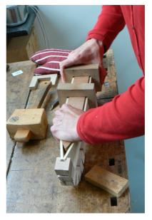
The front, complete with all the cramping blocks, is put in to the fish kettle for an initial steam of ten minutes. Once it comes out, I drive in the cross-wedges as far as they will comfortably go, hitting them with a mallet. Usually they will go in to about three-quarters of their length.
