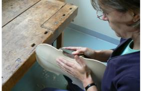
Once the centre joint has dried, you can run round the underside of the front with a block plane to make a flat platform that will eventually be glued to the ribs. This won't of course be completely flat – the area of the top and bottom blocks needs to be built up later with half edging, and you may need to take more out of the Cs than the bouts to get a wide enough flat area for eventual gluing to the ribs.
