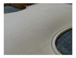
Ray figure is visible over the whole width of the front, not just in the central area.
