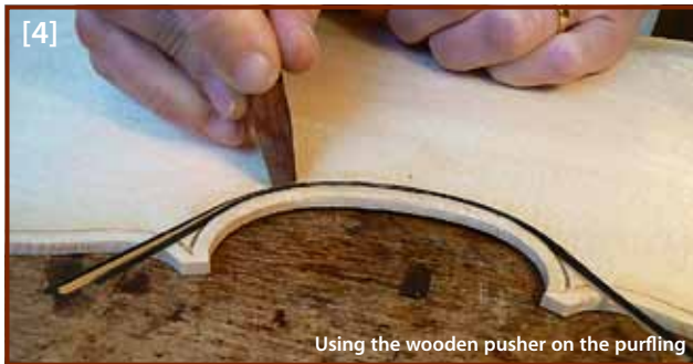
Easing the three purfling strips into the channel
