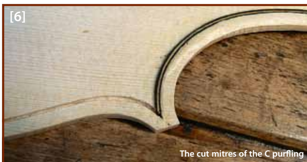
Cutting the purfling to length with a fine-bladed knife
