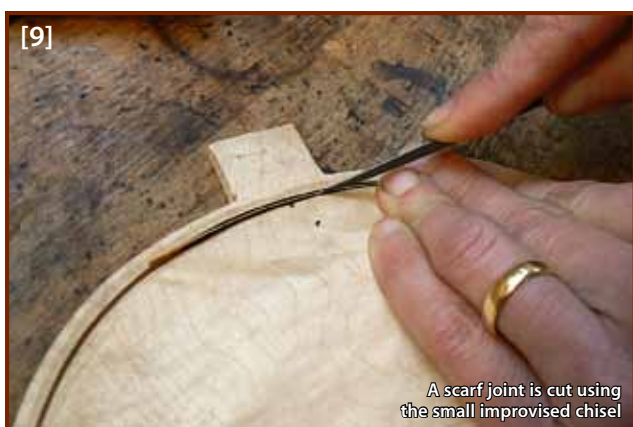
Fitting the three strips of purfling into the glued channel, starting at the corner
