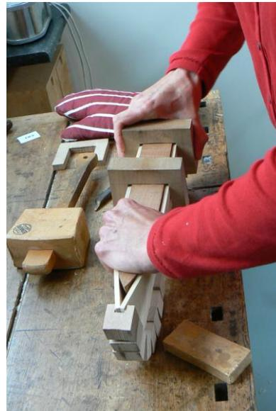
The front, complete with all the cramping blocks, is put in to the fish kettle for an initial steam of ten minutes. Once it comes out, I drive in the cross-wedges as far as they will comfortably go, hitting them with a mallet. Usually they will go in to about three-quarters of their length.
