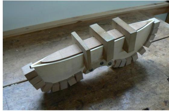
Once all the wedges are in place, the wood is returned to the fish kettle for a last five-minute steam. The wood needs to be steamed in its final form to set the shape. As the wood is cooling all the time that the wedges are being fitted, it is losing its plasticity, so might lose the memory of the final shape once the wedges are removed. By steaming it a final time in its finished state, the wood is “set” and will have the minimum loss of shape.
