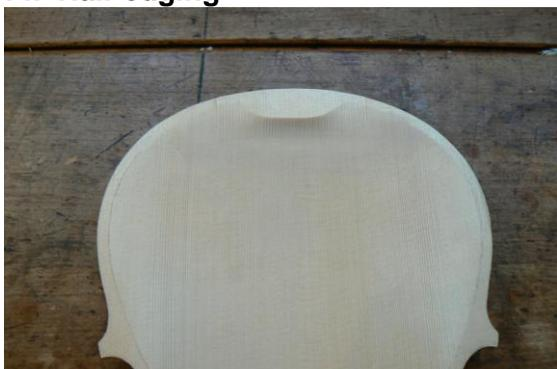
The way the front is bent means that there is not enough wood in the area of the top and bottom blocks to make a flat surface for gluing. So it is necessary to build up these areas by half-edging.
