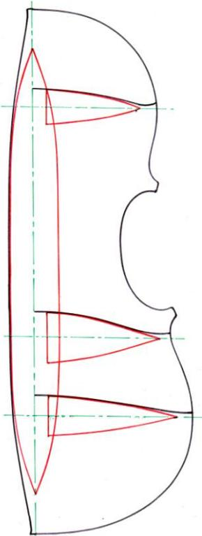
As you can expect the wood to sink once it's been bent and dried, you need to over-bend the wood. I find that a good rule of thumb is to make the width of the "boat deck" wedge at its widest point equivalent to the maximum arching height so that in the central area it follows the external arching of the finished instrument. In effect you're bending the wood to about 5mm higher than the finished instrument.
