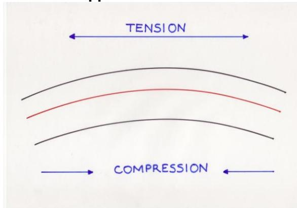
line is in tension, and below is in compression.
