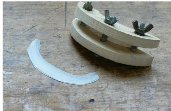
The two halves of the front need to be held together while they are bent. For the upper and lower bouts, I use simple wooden blocks with a 10mm x 10mm slot cut out to receive the wood for the front.
