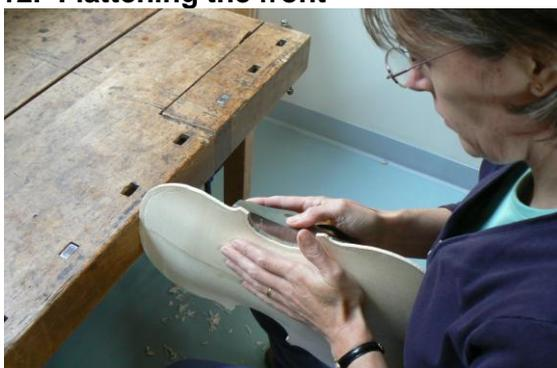
Once the centre joint has dried, you can run round the underside of the front with a block plane to make a flat platform that will eventually be glued to the ribs. This won't of course be completely flat – the area of the top and bottom blocks needs to be built up later with half edging, and you may need to take more out of the Cs than the bouts to get a wide enough flat area for eventual gluing to the ribs.
