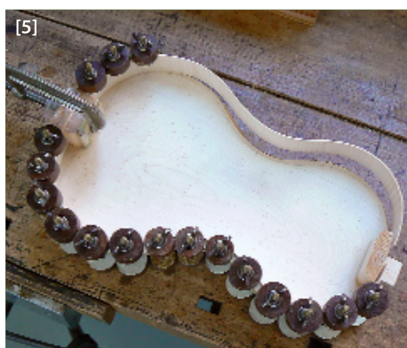
[5] A dry run ensures that everything fits and that the clamps are to hand
