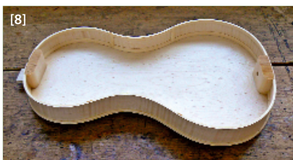
After chamfering and cleaning, the finished rib structure is revealed
