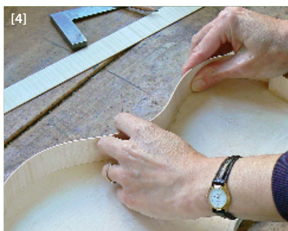
[4] The bent ribs are checked against the back to ensure that they fit
