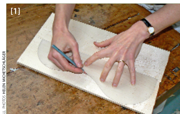
The cornerless viola outline is marked directly from the template
