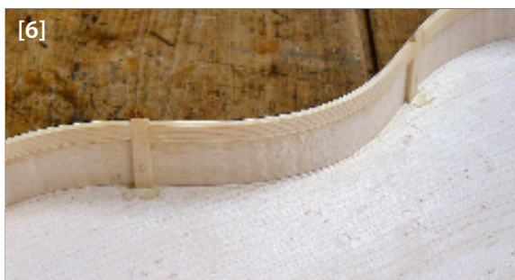
Straps and linings reinforce the ribs at points where they are least curved
