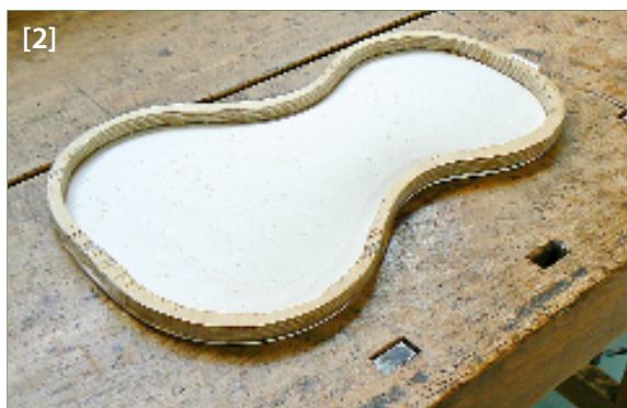
A birchwood jig ensures that the back remains flat while the ribs are added
