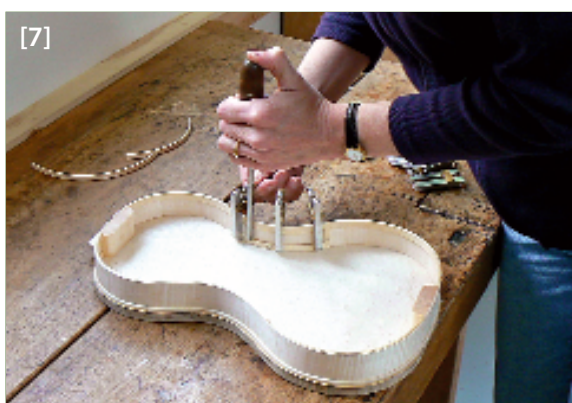
Gluing the lower linings and securing with purpose-made aluminium clamps
